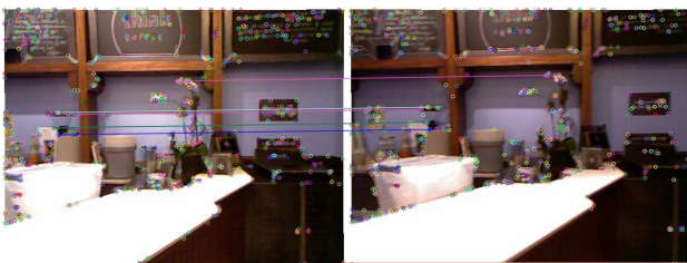
Figure 3. Extract feature points in whole image and good matches condition is 5 times the minimum distance
