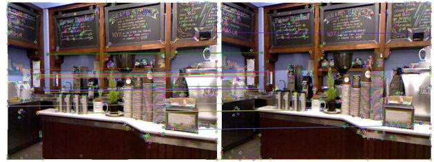
Figure 4. Extract feature points in whole image and good matches condition is 5 times the minimum distance
