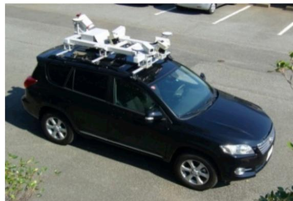
Figure 1. Mobile mapping system
