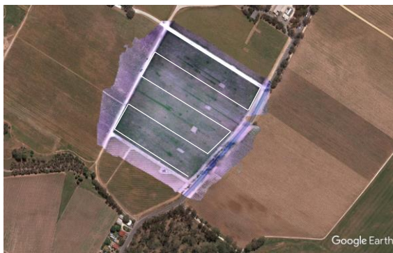
Figure 2: Orthomosaic view of the VIS dense point cloud superimposed onto a Google Earth extract of the Jacobs Creek site at 34° 34' 04" South, 138° 56' 00" East. The white lines depict the approximate ‘lawn mower’ flight.
