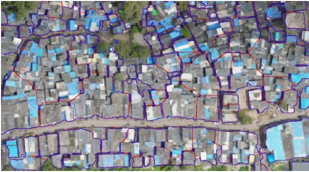
Figure 7.1 Ineffective separation of buildings due to large contact area
