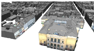
Figure 1. Photogrammetric point cloud aligned with a CityGML model. Facade textures consist of orthogonally projected points.
