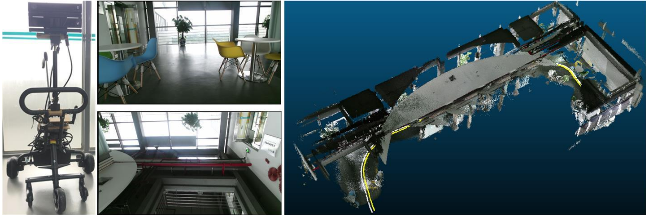
Figure 1. Left: Stereo RGB-D mapping system setup, the two Kinects mounted on a Jetson Tx2, one facing upwards and the other one facing downwards. Middle: Camera views of two camera at the same time-stamp. Right: The built dense point cloud using the two Kinect
