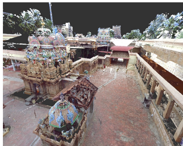
Figure 13. TLS of shrine at Nageshvara temple, Kumbakonam
