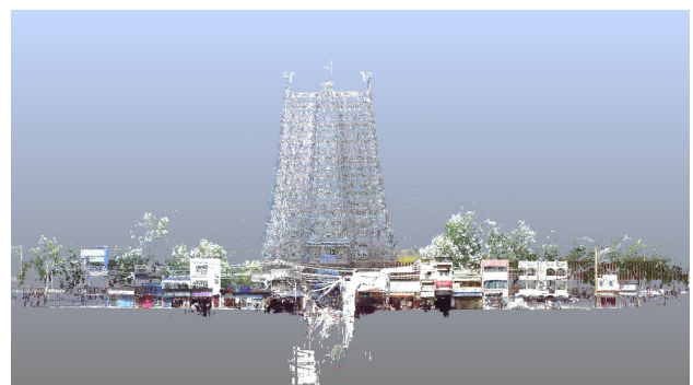
Figure 6. Orthophoto of TLS showing front elevation of Western gate of Minakshi temple, Madurai, India
