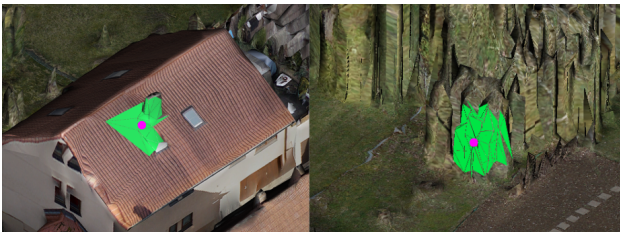
Figure 2. SPNHs (radius 1.5 m, green) and corresponding COGs (pink) for which the feature vectors are generated.
