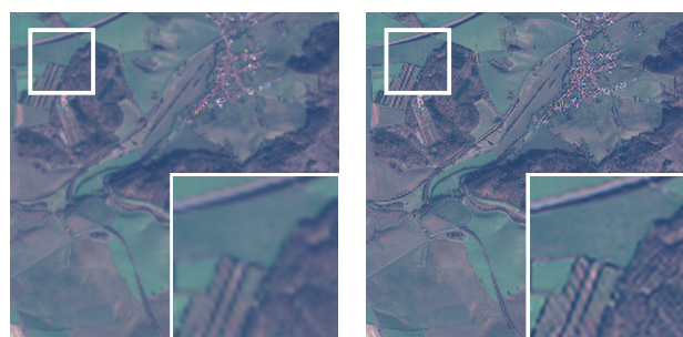
Figure 1. RGB composites with a spatial resolution of 10 m, up-sampled by a factor of two using bilinear interpolation (left) and our deep residual learning SISR approach (right).
