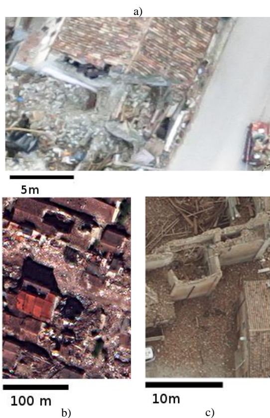
Figure 1 Examples of damaged and undamaged regions in a) UAV (Pescara del Tronto, Italy, 2016), b) satellite (WorldView 3, Amatrice, Italy, 2016) and c) manned aerial vehicles (St Felice, Italy, 2012) imagery.
