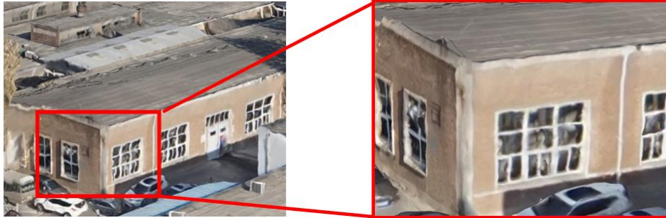
Figure 7 The model constructed only by the oblique photogrammetry
