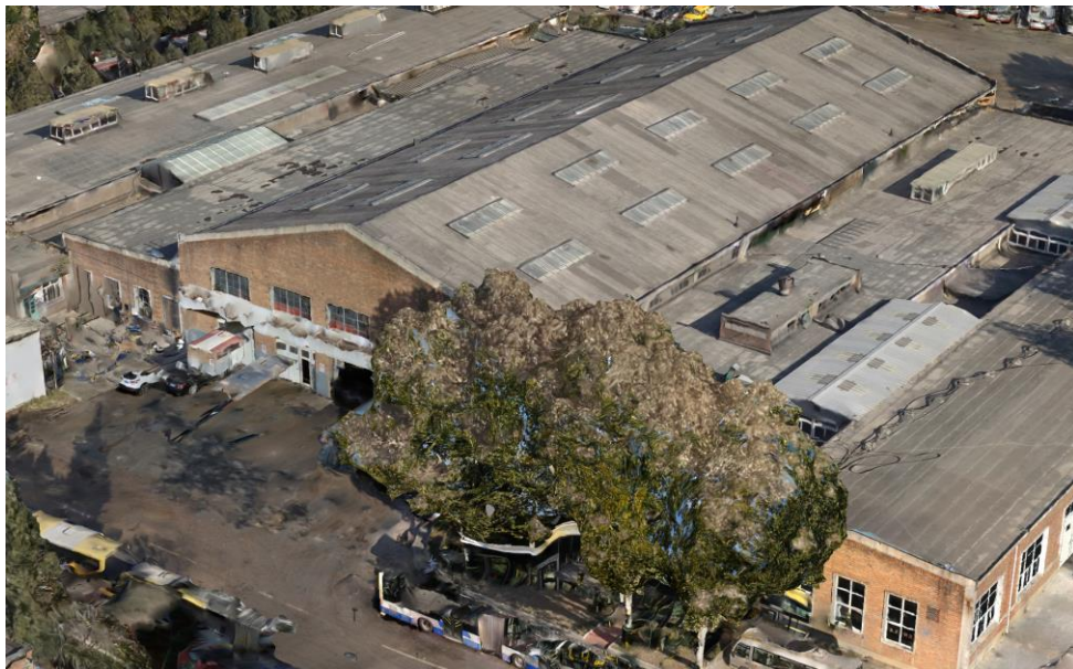
Figure 10 The big experiment area model produced by the oblique photogrammetry and the close range photogrammetry
