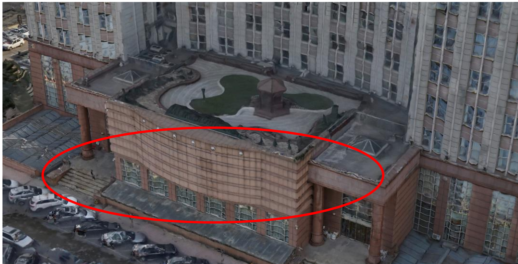
Figure 13 The air view of one big building model produced by OP and close range photogrammetry
