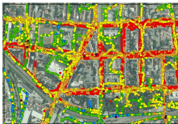
Figure 8. Classified measurements displayed in QGIS (blue and green dots represents lowest noise levels, red and purple the highest) (Vuković, 2015)
