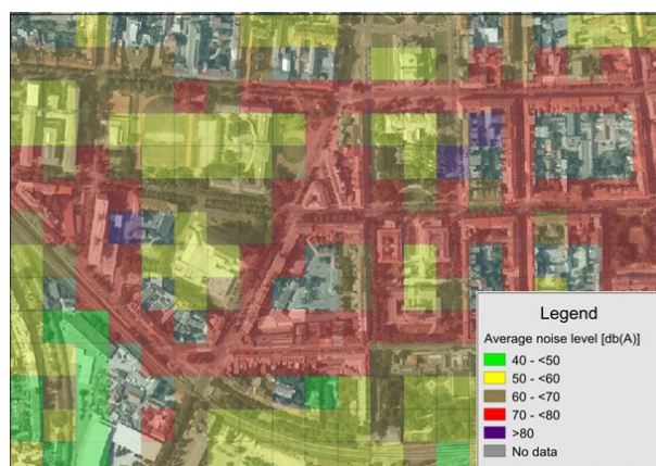
Figure 9. Representation of calculated average noise level displayed in QGIS on digital orthophoto (Vuković, 2015)
