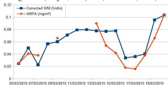
Figure 2. Calibration of the dust sensor.
