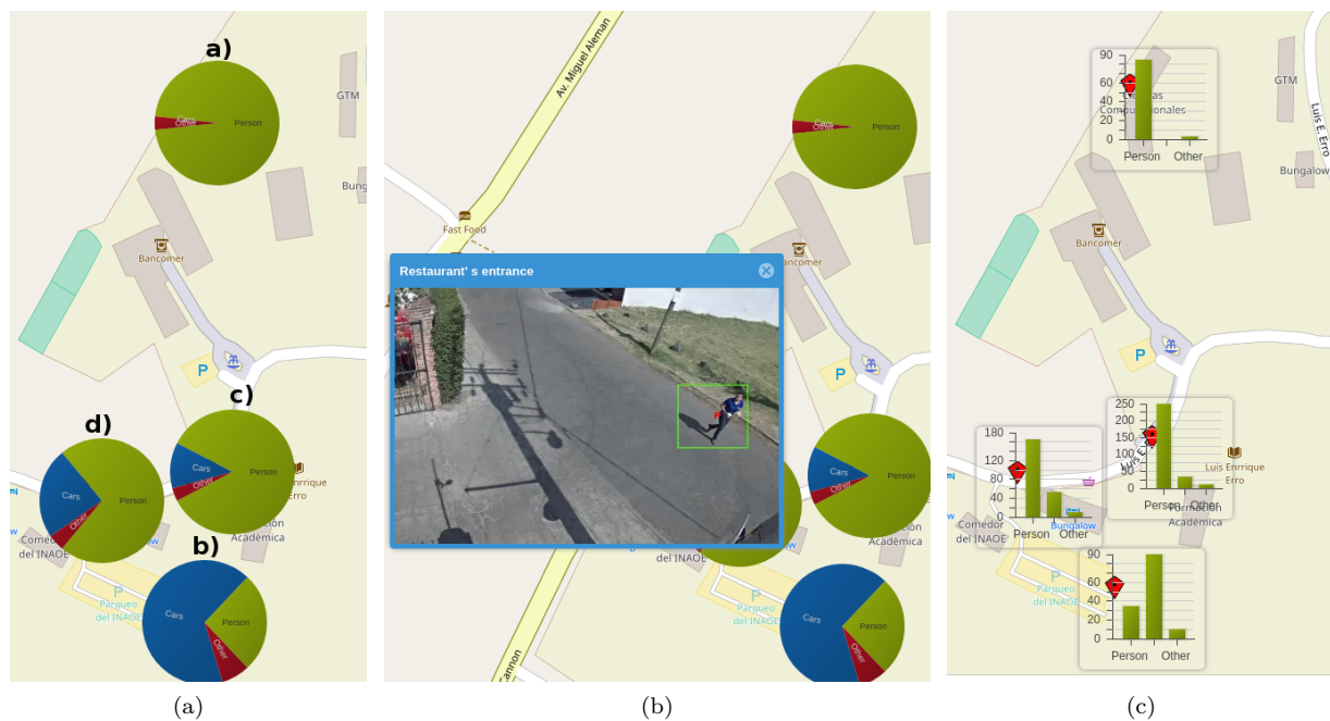
Figure 5. Resulting visualization of the number of persons (green), vehicles (blue), and others (red) detected by each camera during two hours (see queries 1, 2, and 3). Left figure shows a Pie-chart visualization. Center figure shows a Pie-chart visualization and real time video rendering of camera d). Right figure depicts a Bar-chart visualization. In this figure is shown that camera a) does not recognize vehicles because it is in an indoor scenario. Cameras c) and d) have a considerable amount of persons because it correspond to the lunch time. Finally, b) camera has a lot of vehicles because it is in the parking lot (best seen in color).
