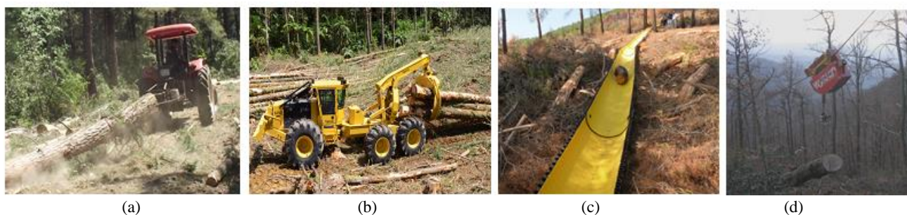
Figure 1. Primer forest transportation methods used in Turkey: a) Farm tractor, b) Skidder, c) Cable system, d) Chute system
