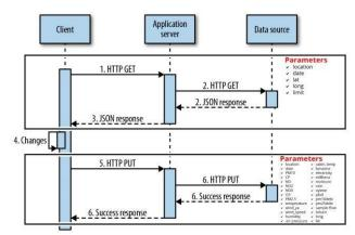
Figure 4.AQ Web API Sequence Diagram
