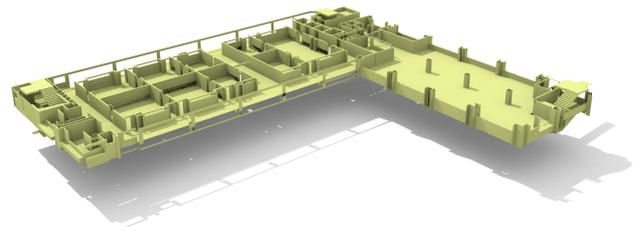
Figure 1. CityGML dataset obtained from IFC (storey of one building) with the approach developed within our project. Source of the input IFC dataset: BCA Singapore.
