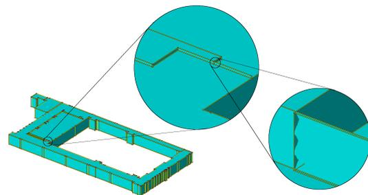
Figure 3. Self-intersecting ring in a complex geometry item, present in both original IFC and generated CityGML
