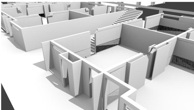
Figure 2. Walls as constructive elements instead of semantic surfaces (the same dataset as in Figure 1). These are supported in the future CityGML 3.0, but may conflict with the well ingrained semantic surface concept in 3D GIS. The image also shows overlap between geometries.
