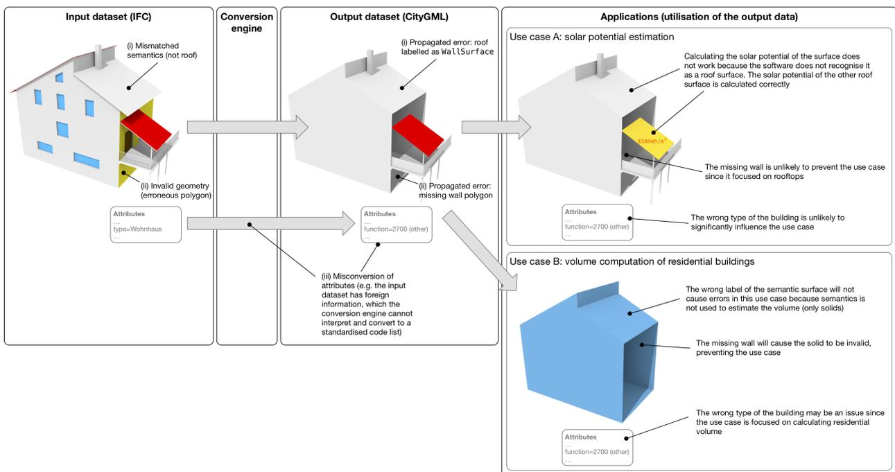
Figure 4. Combination of different types of errors results in multiple categories that are depending on the use case context. These errors are further described in Table 1. Source of the dataset (with modifications) used to generate the illustration: Institute for Applied Computer Science, Karlsruhe Institute of Technology (Häfele, 2011).
