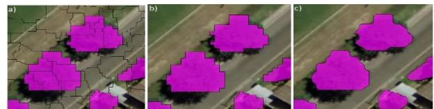
Figure 8. Resizing the classified objects, a) Image showing segments before merging b) Image showing segments after merging c) Image showing result of resizing of merged segments using pixel-wise object resizing (growing and shrinking) algorithm.
