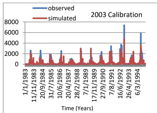
Figure 18 Line graph showing simulated and observed runoff vs time at daily time step for the year 2003 (calibration)
