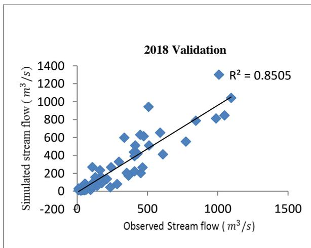
Figure 15 Plot showing simulated vs observed runoff at monthly time step for the year 2018(Validation)
