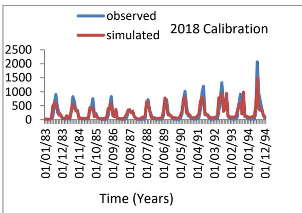
Figure 22 Line graph showing simulated and observed runoff vs time at monthly time step for the year 2018 (calibration)
