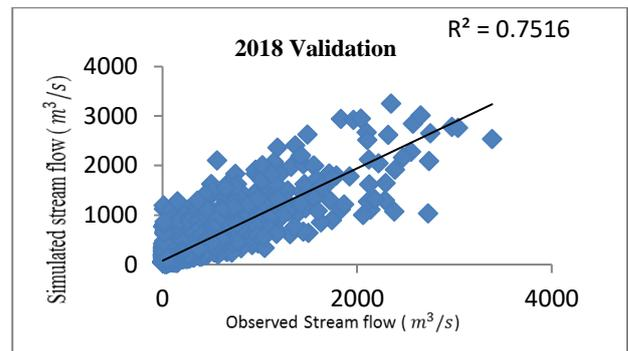
Figure 17 Plot showing simulated vs observed runoff at daily time step for the year 2018 (Validation)
