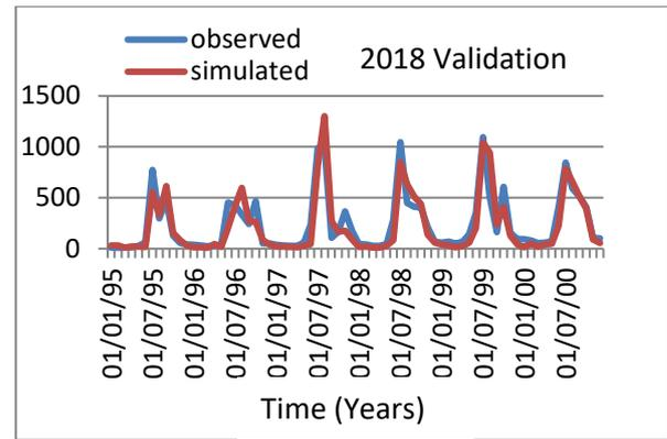
Figure 23 Line graph showing simulated and observed runoff vs time at monthly time step for the year 2018 (validation)
