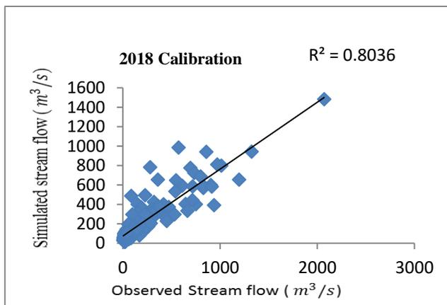
Figure 14 Plot showing simulated vs observed runoff at monthly time step for the year 2018(Calibration)
