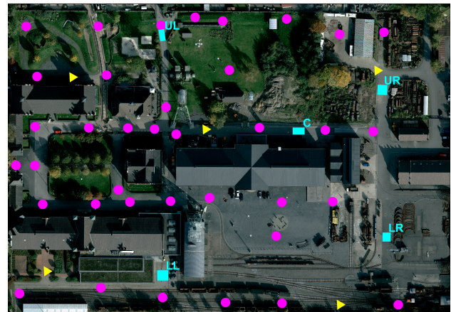
Figure 2. Orthophoto of test field Zeche Zollern with GCP (yellow triangle)/Check point (magenta circle) distribution and areas of surface analysis (cyan rectangle)
