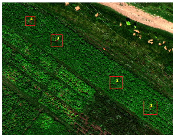
Figure 10. Orthophotomosaic on December 28 1:25PM, with identification of areas of surface elevation change due to individual plants removal
