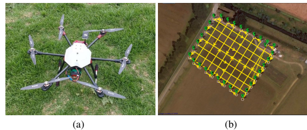
Figure 2. UAV used and flight mission. (a) Hexacopter Tarot 680 PRO; (b) flight mission.
