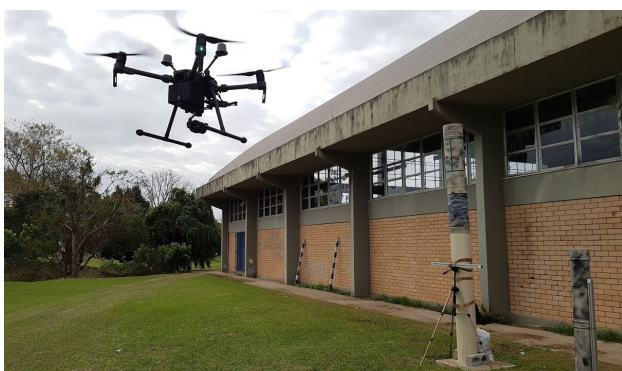
Figure 14. Experiment setup. RPA during acquisition of images of a PVC pipe (riser simulacrum) for photogrammetric measurement.
