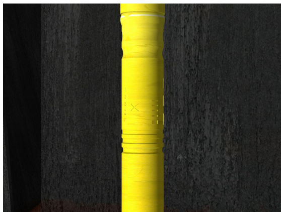
Figure 9. Sample of acquired image. The riser diameter is of about 300 mm. Some included riser artificial defects and artifacts; Camera FoV of 2.0 m x 1.5 m.
