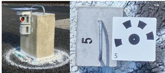
Fig. 2: The structure of the marker with the prisms: left side view: the centres of the three elements are arranged collinearly, the distances are known. Right: marker in aerial view.
