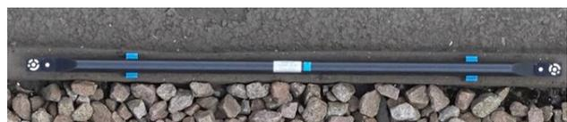
Fig. 9: Highly accurately calibrated CFRP scale for checking the local image scale
