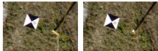
(a) Orthoimage by using NN (b) Result of SR-O
