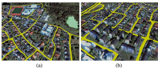
Figure 5. 3D view of the refined DSM model textured by the orthophoto and road segmentation.
