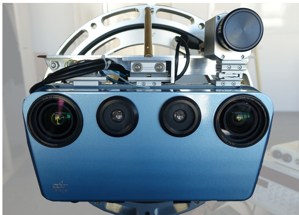
Figure 3. Stereo-Camera system with long-wave infrared camera attached on top. The system is mounted on a rotary plate for calibration purposes.
