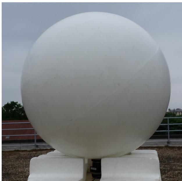
Figure 13. Implementation of flat-field calibration using the spherical diffuser.
