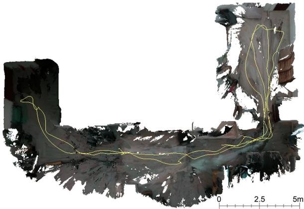
Figure 2. Multi-room reconstruction and the trajectory estimated by the proposed system.
