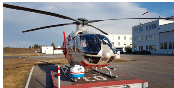
Figure 3. DLR 4k camera system mounted on the fuselage of a EC135 helicopter.
