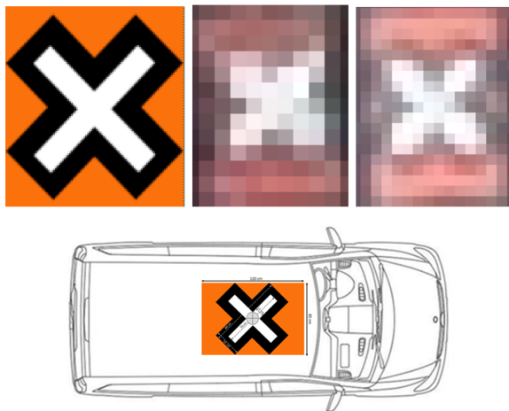
Figure 6. Magnetic sticker with cross installed on vehicle roof (1.2 m × 0.85 m). GNSS antenna is installed in the center of the cross. Top left: original resolution, top middle: imaged with 10 cm GSD, top right: imaged with 7 cm GSD.
