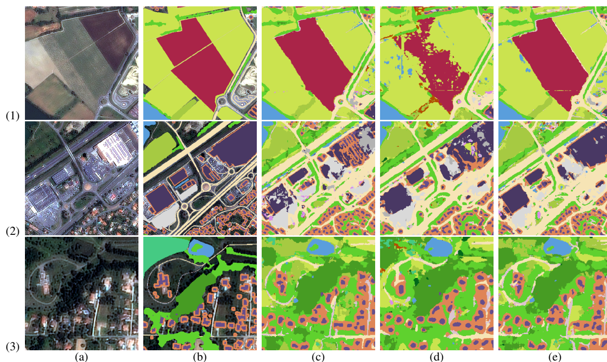
Figure 3. Rows : (1) Vineyards, (2) Industrial and commercial area, (3) Paths in diffuse urban area. Columns : (a) SPOT image, (b) Ground truth, (c) SPOT inference, (d) S2 inference, (e) Fusion inference
