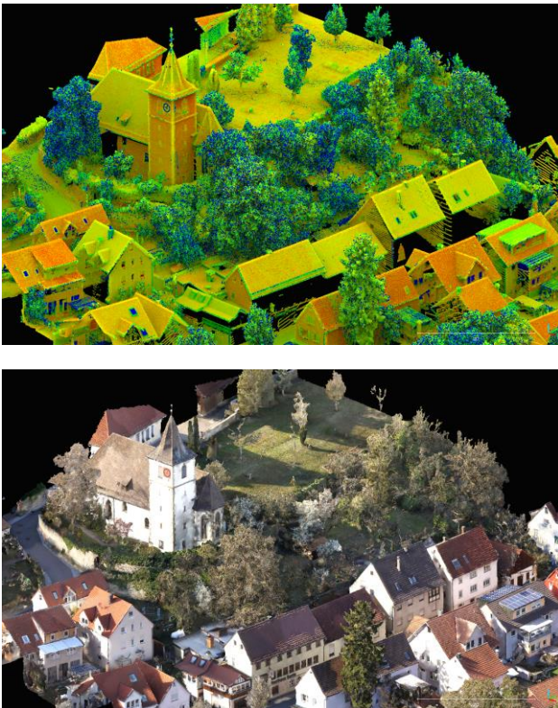
Figure 9. LiDAR point cloud with corresponding colour coded reflectance (top) and 3D mesh with corresponding image texture (bottom).
