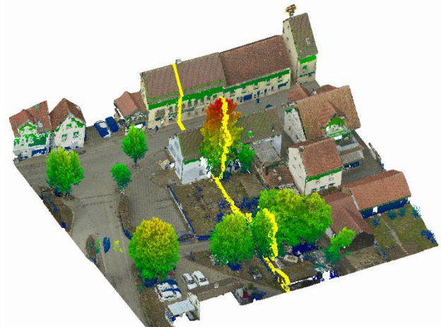
Figure 7. Comparison of 3D points from MVS (RGB) and LiDAR measurement (height coded). Yellow line defines profile depicted in Figure 8.
