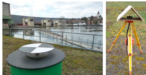
Figure 2. Ship lock and photogrammetric control point (PCP) on a pillar (left), LiDAR control plane (LCP) (right).
