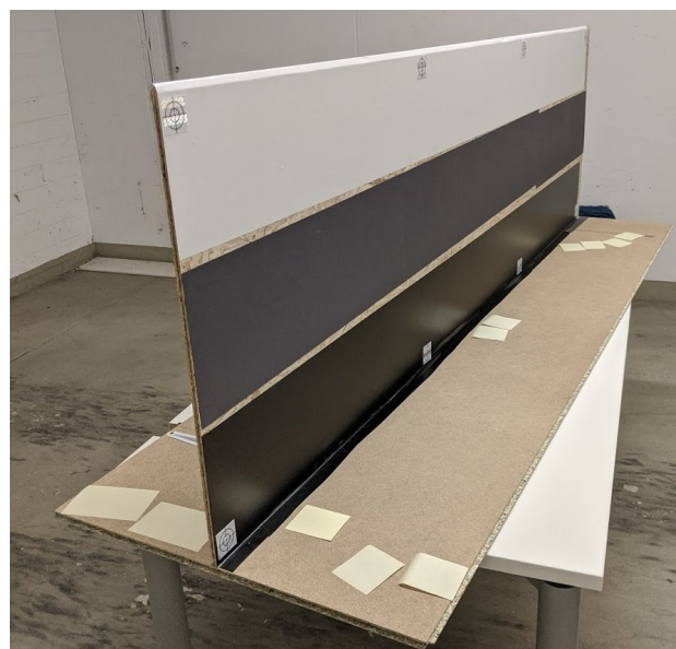
Figure 2. Wooden board with white, grey and black surface materials. The reflective tape markers along the edges are used for the tachymetry. The image shows the board at an offset of approximately 20^\circ with respect to the ranging direction. Refleactions can be seen in the black surface, indicating that the surface is not Lambertian.
