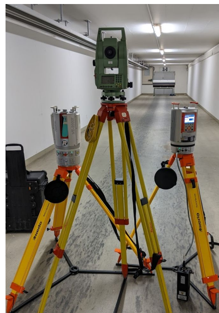
Figure 1. Measurement setup. Left: RIEGL VZ-2000i , center: Leica TCRA705power , right: RIEGL VZ-400 . In the background, the experiment board can be seen at a range of 30 m. The experiment was carried out in a basement which allows a maximum target range of about 250 m.
