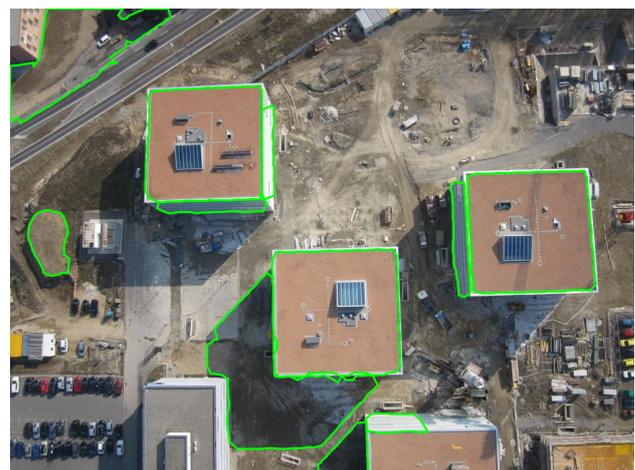
Figure 9. Polygonal contouring. Using a basic edge tracking procedure as subsequent step to our method (see text), one can extract the contours of a specific class of objects (here building roofs) as low complexity polygons (green curves). Even if we note some errors, most of roofs are correctly polygonalized with such a basic tracking procedure.
