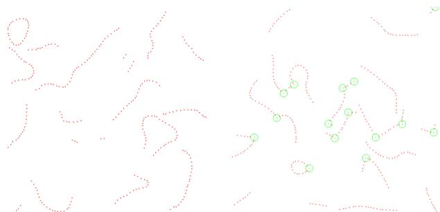
Figure 6. Point distribution simulated with an alternative geometric prior. Our shape prior can be completed by an additional term that favors smooth (left) and piecewise-smooth (right) angles between successive Delaunay edges. Points are then distributed regularly along curves. This complementary prior can be used for extracting free-form object contours.
