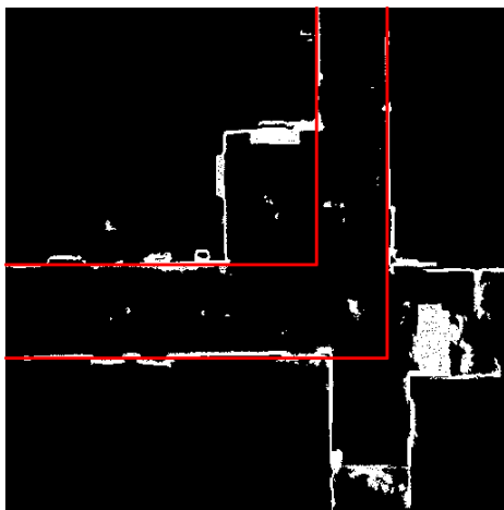
Figure 5. BIPC and the extracted corridor, where walls are in white and the corridor is in red.
