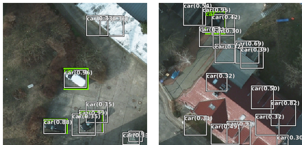
(b) Detections of the model trained with 1000 generated images only. A lot of false positive detections are visible; however, the true positive detections are quite accurate.
