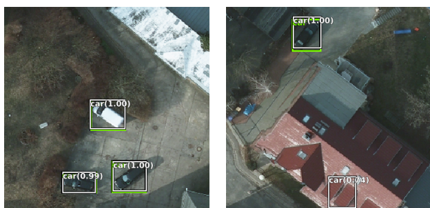
(d) Detections of the model trained with 1000 generated images and 32 real-world images. The model produces no false positives in the left image, and in the right image, only one false positive is still visible.
