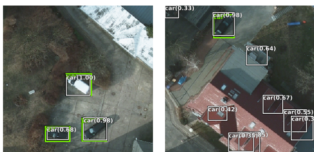
(c) Detections of the model trained with 1000 generated images and eight real-world images. The model produces no false positives in the left image, and in the right image, much fewer false positives are visible.
