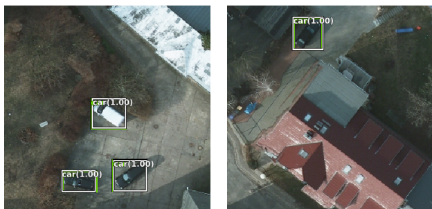
(a) Detections of the baseline model trained on the complete real-world data set. The detections are quite accurate and have high confidences; no false positives are visible.
