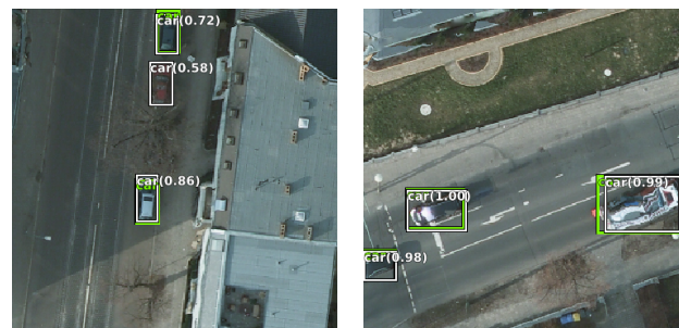
Figure 9. Left: An example of detections of hidden vehicles: the detection of the car in the middle has no corresponding annotation, which counts as a false positive; the detection of the lower car is better than the annotation, which may also impact the AP negatively. Right: An example of a detection of a fragmented vehicle.
