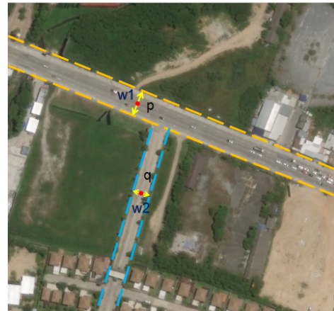
Figure 3. For pixel p and q, the width of which ( w_1, w_2 ) is calculated along the direction perpendicular to road direction.
