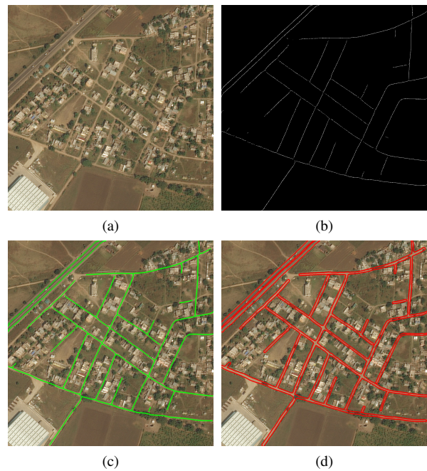
Figure 5. Extraction of centerlines and edge lines. (a) Input image. (b) Binary map for centerlines. (c) Tracked road centerlines. (d) Extracted road edge lines.
