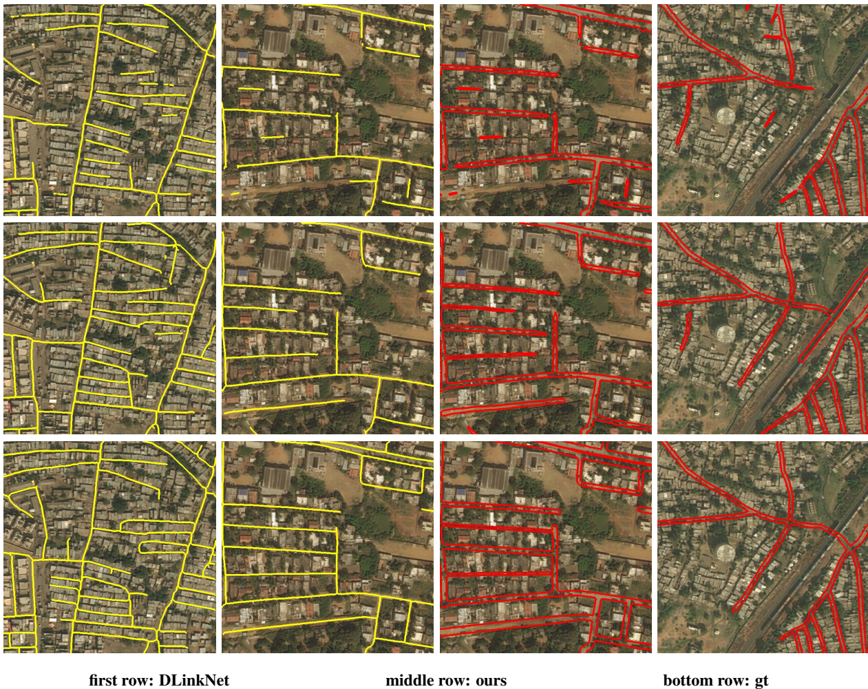
Figure 8. Examples of road extraction results on the DeepGlobe and SpaceNet datasets. The first row shows road centerlines and edge lines extracted by DLinkNet, the middle row shows results of the proposed method and the bottom row shows the ground-truth. We overlaid the extracted road centerlines(yellow) and edge lines(red) on the image. Our approach extracts more complete road network while has lower error rate than other methods.
