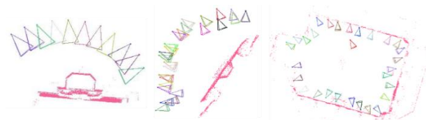
Figure 7. Visualization of benchmarks’ SfM results by “HM” (after bundle adjustment). Colourful triangles denote exterior pose parameters; red dots are estimated 3D object points.
