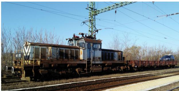
Figure 1. For technical reasons, the *Riegl VMX-450* MMS sensor was mounted on a car, which was placed on a carriage.
