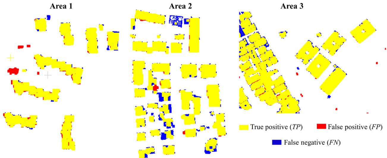
**Figure 9.** Visualization of building detection result at the per-pixel level for areas 1, 2 and 3. Yellow color represents true positives (*TP*) (building correctly detected), red represents false positives (*FP*) (incorrectly detected as building), and blue corresponds to false negatives (*FN*) (omitted buildings).
