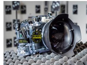
(b) Camera system for close-range data set. A Nikon D750 with 24mm lens in a NiMAR NI3D750ZM housing with dome port
