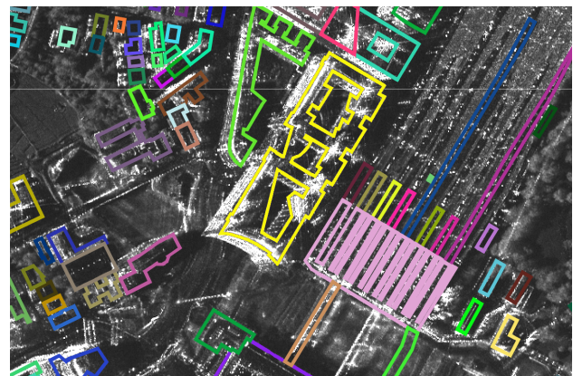
Figure 2. A sample of the geocoded "HighRes SpotLight 300MHz" scene over Stuttgart, Germany (orbit cycle 119, spot 076). Overlaid with OSM building footprints. Each building instance in a different colour. The original 10 \text{ km} \times 9 \text{ km} wide scene contains more than 38000 OSM building footprints.
