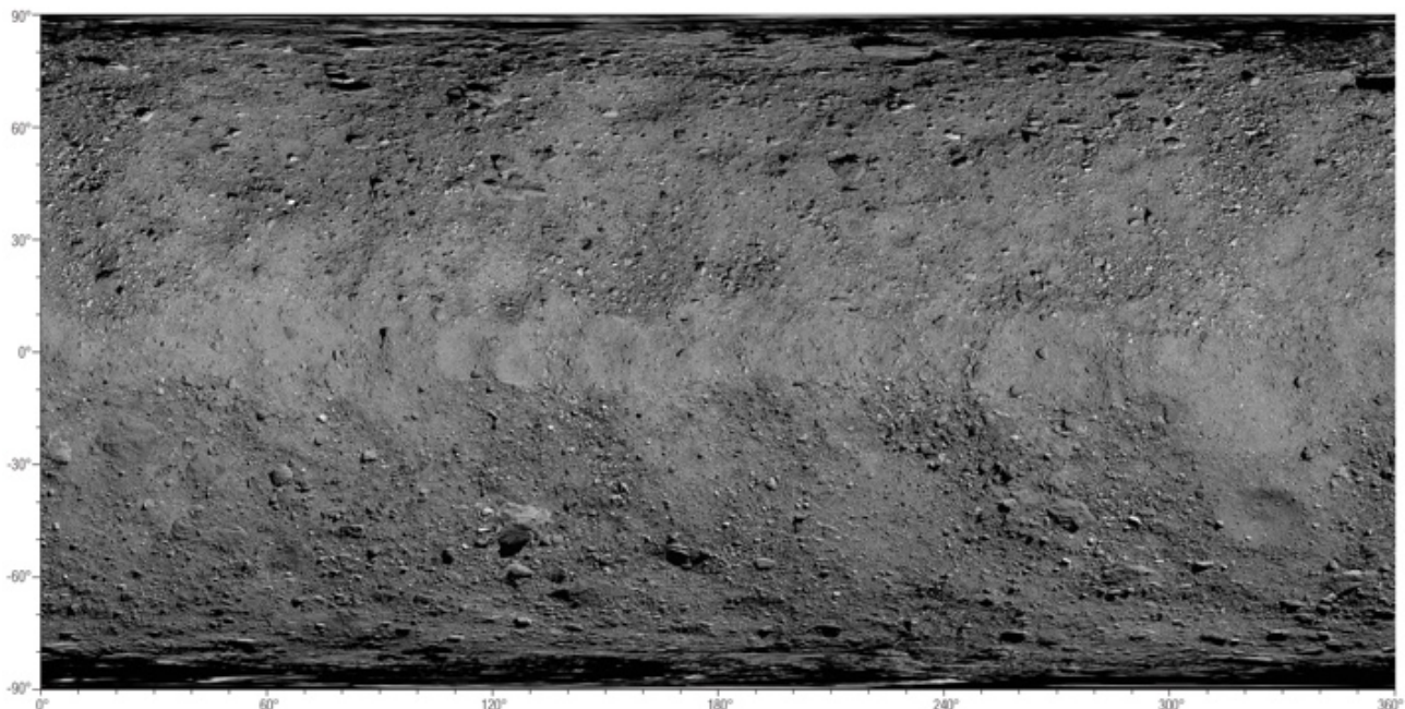
Figure 5. Global panchromatic basemap of Bennu created from 2155 OCAMS PolyCam images acquired at a pixel scale of \sim 5 cm (Bennett et al., 2020). Projection is equirectangular.
