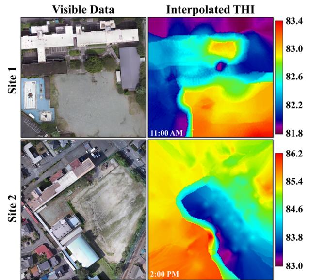
Figure 7. Spatial distribution of the THI interpolated from point vectors collected during the ground surveying.
