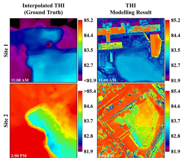
Figure 9. THI modeling result for site 1 and site 2 implementing the random forest regression (Note that site 1 is at 11:00 AM and site 2 is at 2:00 PM). The scaling and the color bar is synchronized for the interpretation purpose.
