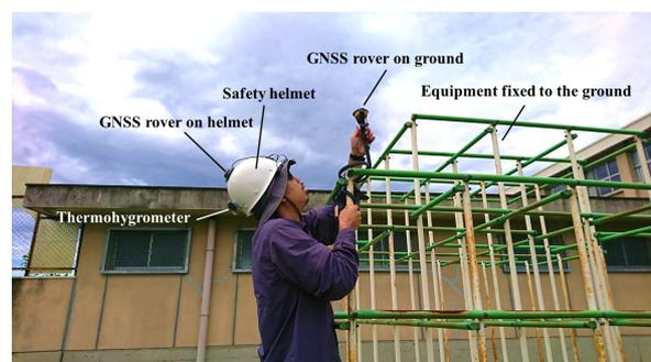
Figure 5. Equipment to collect ground truth data for THI.
