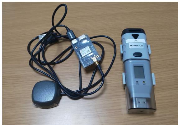
Figure 3. GNSS equipment (left) and thermohygrometer (right).
