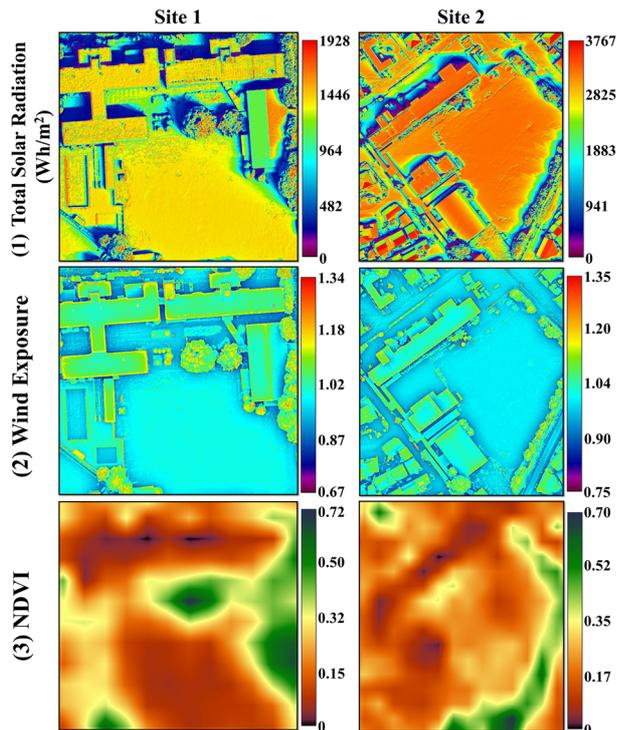
Figure 8. Explanatory variables for the (1) Total solar radiation ( $\text{Wh/m}^2$ ), (2): Wind exposure, (3): NDVI for (left) Site 1 and (Right) Site 2. Solar radiation shown here is only the total radiation for the visual purpose. Note that site 1 is modeled up to 11:00 AM, while site 2 is modeled until 2:00 PM for solar radiation.
