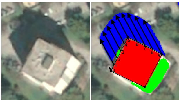
Figure 9. Left: input image, right: predicted masks for rooftop, facades, shadow, and shadow rays to compute shadow length.
