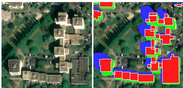
Figure 2. Example ground truth masks. Red: rooftops, green: facades, blue: shadows, white: contours/walls.
