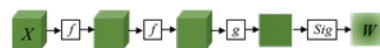
Figure 7. The workflow of our attention generation, i.e., the PSA module, where X , f , g , Sig , W denote the feature map, 3 \times 3 convolution, 1 \times 1 convolution, the Sigmoid activation function and the attention.
