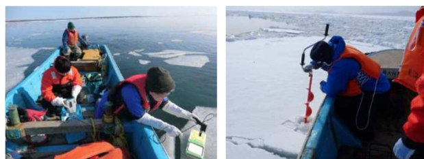
(a) Reflectance measurement (b) Ice thickness measurement Figure 3. In-situ measurement from a vessel.
