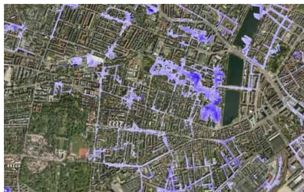
Figure 3. Example of city cloudburst flood as simulated by 2D model (Copenhagen)
