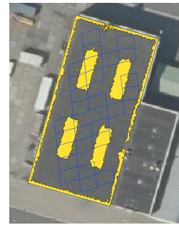
Figure 10. Example of a visualization obtained during the validation. Mapped ‘deviations’ are shown in yellow and can be overlaid with the (modified) pixels resulting from hyperspectral imagery pixels and contained in the building roofprint (geometry in blue). Settings used: distance threshold 20 cm and angular threshold 2°.
