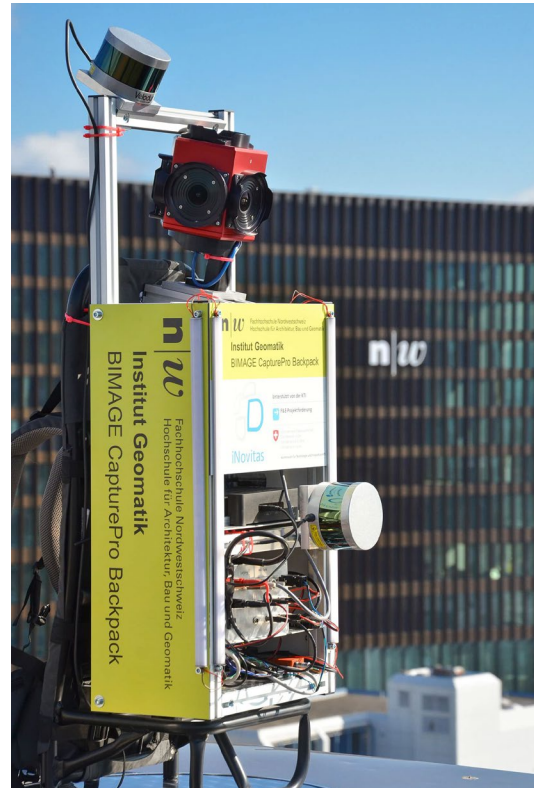
Figure 3. Mobile mapping system (Backpack) developed by FHNW, Institute of Geomatics (Blaser et al 2018)
