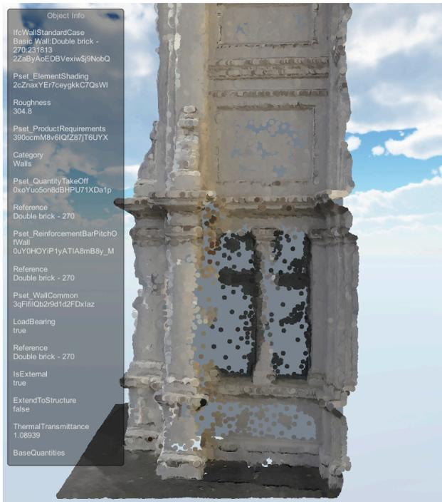
**Figure 3.** The point cloud of a wall building element after the point cloud cutting function is performed. Only the left-hand side of the split-screen is shown.
